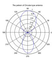
Figure 3(c). Radiation pattern by the DDE algorithm in the NLOS case
