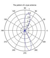
Figure 2(a). Radiation pattern by the GA algorithm in the NLOS case (a) L shape array
